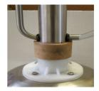
Using hot water fit the rubber sleeve to the thermometer leaving only the red bulb Protruding (this may be pre-fitted).
